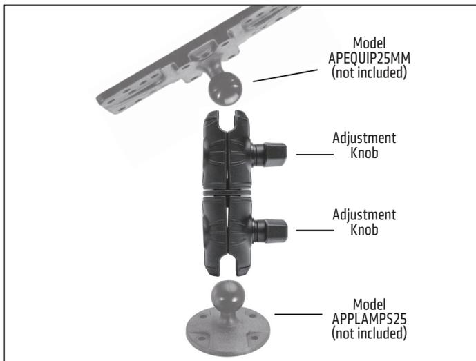
**2** To swivel the shaft arm, loosen the top or bottom adjustment knobs and rotate the arm to the desired position. Retighten knobs to set.
